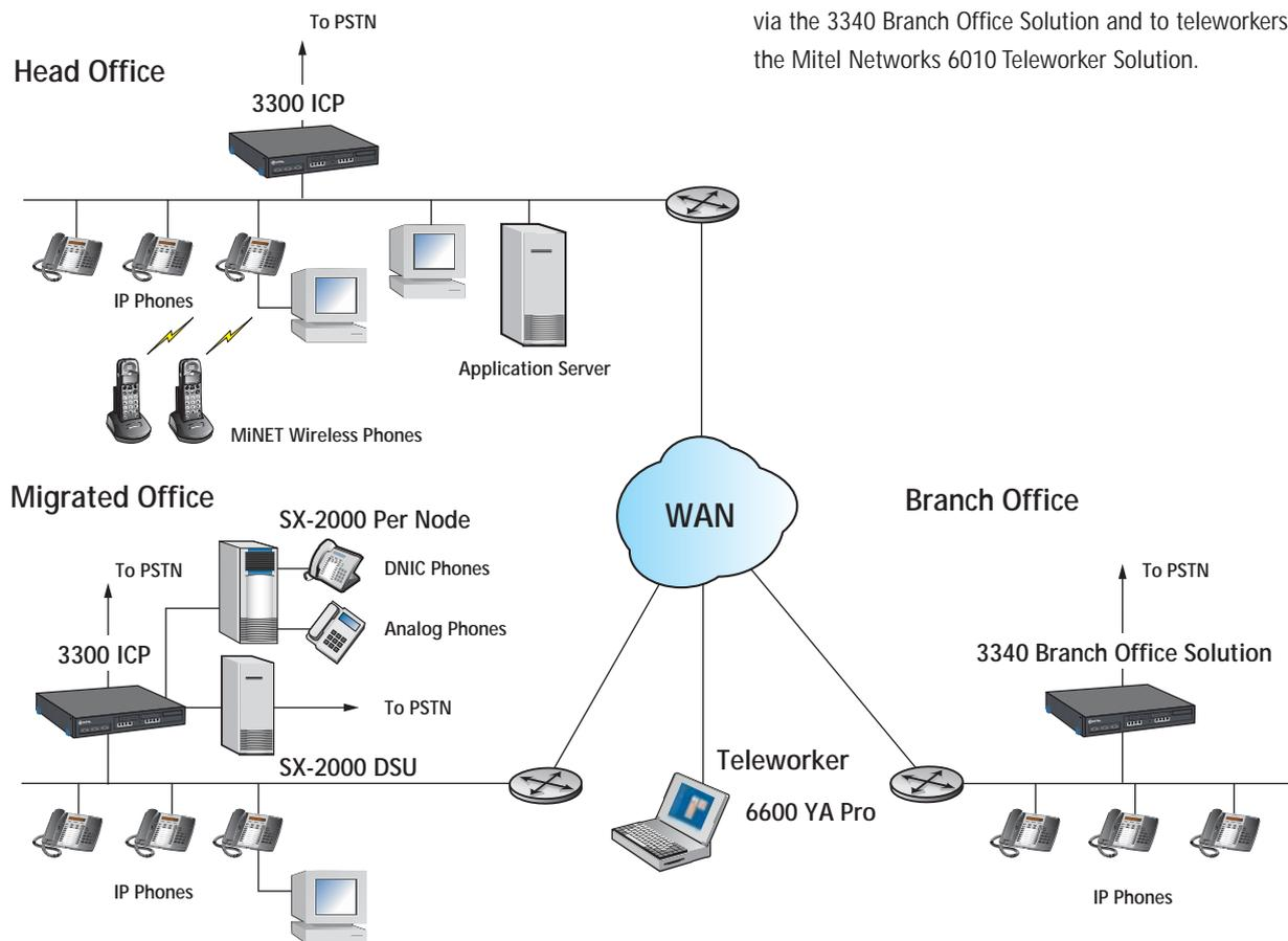
The 3300 ICP is a resilient solution that supports single and multiple location enterprises, with IP networking extending full head office capabilities to the branch office via the 3340 Branch Office Solution and to teleworkers via the Mitel Networks 6010 Teleworker Solution.
